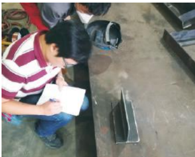
焊缝表面检测 Visual Inspection at welding line
