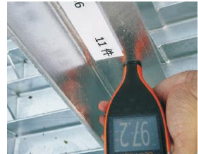
材料镀锌涂层检测 Detecting for hot-dip galvanized coating
